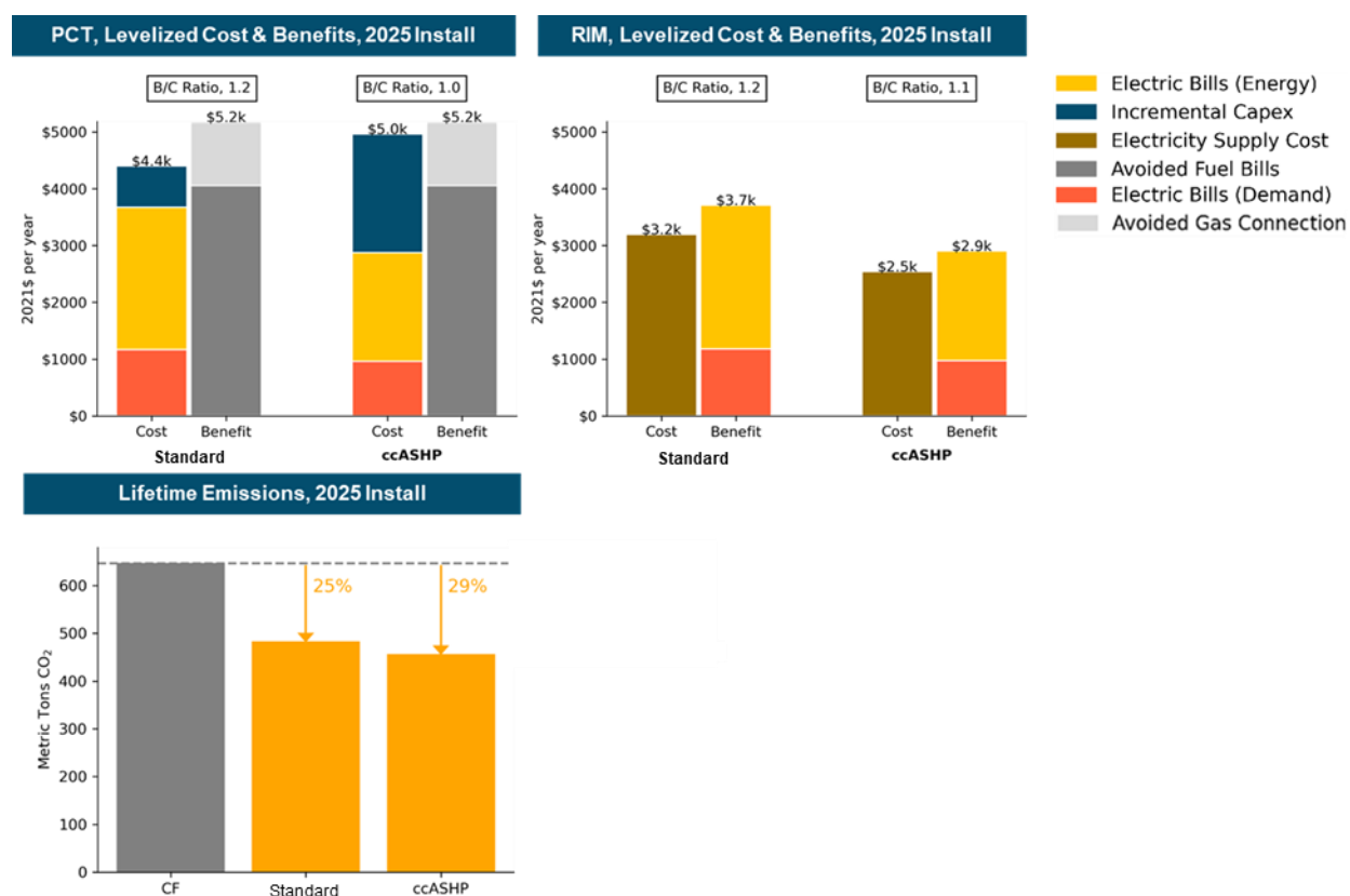
Figure 2-19. Small Office New Construction HVAC Electrification, IPL
