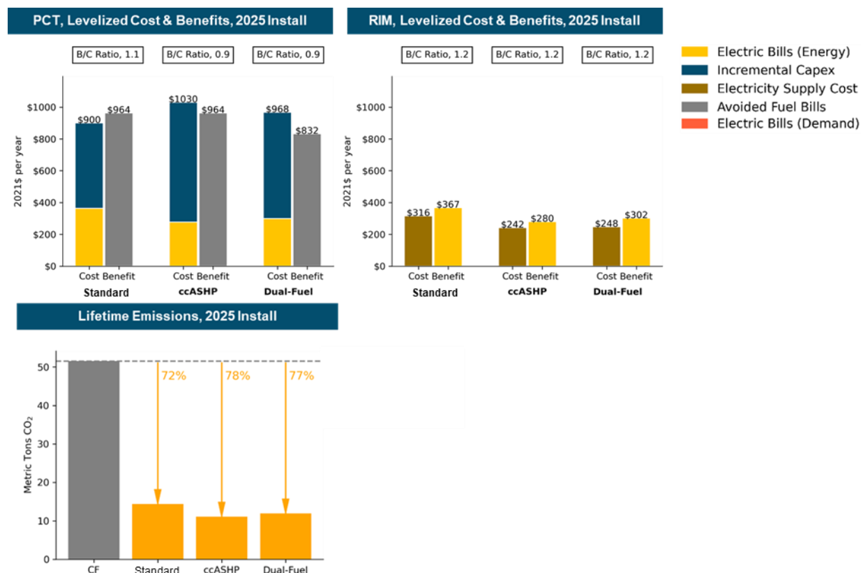
Figure 2-13. Single-Family Residential Retrofit HVAC Electrification for Delivered Fuel, 2025 Installation, Tacoma Power
