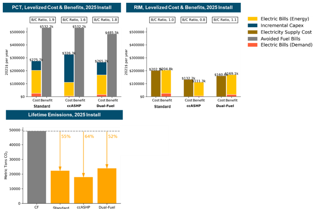
Figure 2-18. Large Healthcare Retrofit HVAC Electrification, Tacoma Power
