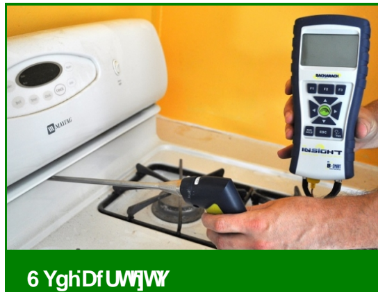
Test gas oven for carbon monoxide using a combustion gas analyzer
