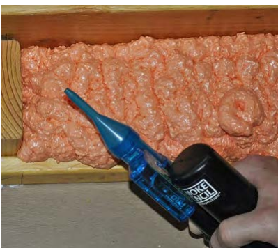
Whatever option chosen, test with chemical smoke at 50 pascals of pressure difference to verify no leakage
