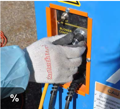
Adjust machine settings for loose fill: open gate for high material flow, allow enough air pressure to avoid clogging.
