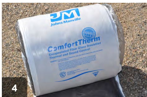
Select appropriate batt thickness and R-value. Wrapped batts provide a built in vapor barrier
