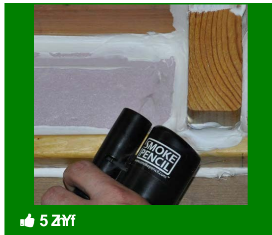
Whatever option chosen, test for visible air movement with chemical smoke at 50 pascals of pressure difference
