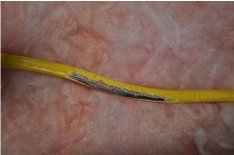
Check for frayed or worn electrical wires
