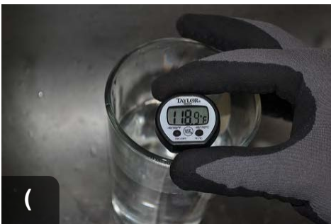
After adjustment and insulation, retest to verify temp is under 120 degrees
