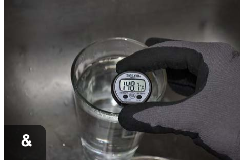
Hot water temperatures should not exceed 120 degrees Fahrenheit
