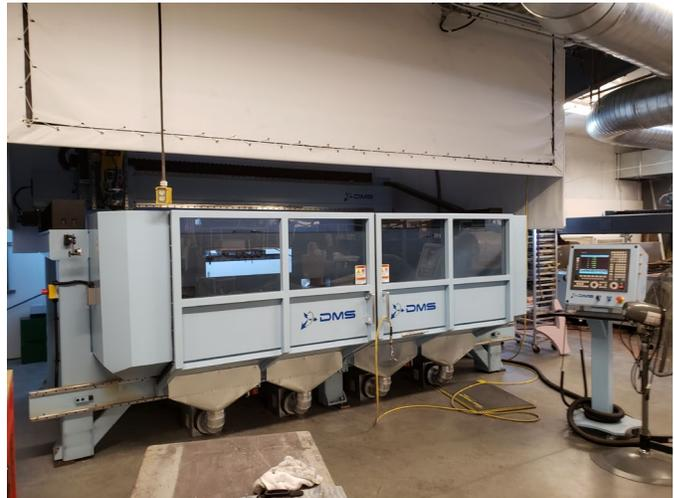
The primary issue with the machine (aside from added dust control) was in alignment of the gantry and machine ways. We learned after the fact that this was an issue with DMS machines and once the warranty and service approaches were exhausted with DMS we had to contract out for this effort. The re-alignment and finishing was successful and the machine is at full operational capability.
