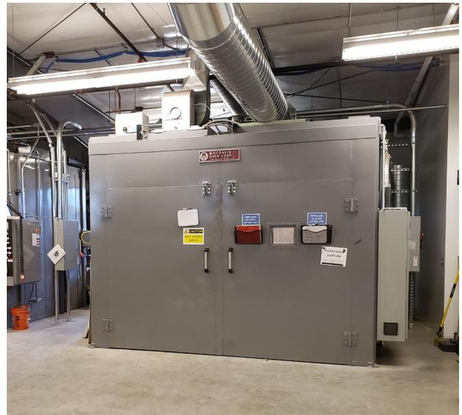
The key issue encountered with the oven has been quality of electric service, since the local service apparently has been causing fuses to burn out at much too high a rate. Several custom fixtures and racks for part cure have been made at CRTC over the last couple years, allowing more efficient loading and unloading as we typically cure overnight off the day's production.
