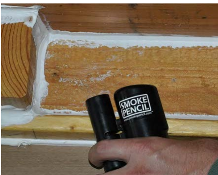
All Options: Test with chemical smoke at 50 pascals of pressure difference to verify no air movement
