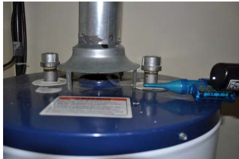
Complete spillage test using chemical smoke pencil
