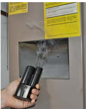
Complete spillage testing on all combustion appliances
