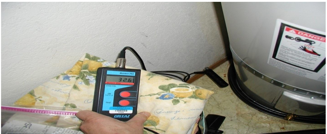
Figure 11. Plumbing leak: Hot water tank leaked and was replaced, but wallboard is still sopping wet (meter says 32.6; 28 is very wet) and mold will grow. This is where a moisture meter comes in very handy; finding damp materials adjacent to a leak before mold grows saves time and money for landlords...the meter may well “pay for itself.” This wet drywall, IF it can be saved, needs to be opened and aggressively dried using professional dehumidification techniques.
