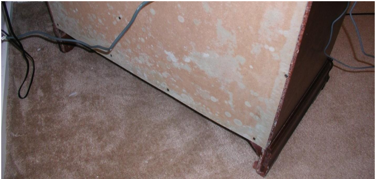
Figure 4. Condensation: Tenants kept the apartment at 60 degrees, cold enough that the back side of their dresser was below “dew point”, the temperature at which typical moisture levels in the air will condense on a surface. With the dresser chronically wet, mold got started and amplified. This can probably be scrubbed off (outside!) and painted. To prevent a recurrence of the mold, surfaces need to be kept warmer either by increasing the apartment temperature and/or allowing air circulation behind the dresser, or lowering the relative humidity in this space.
